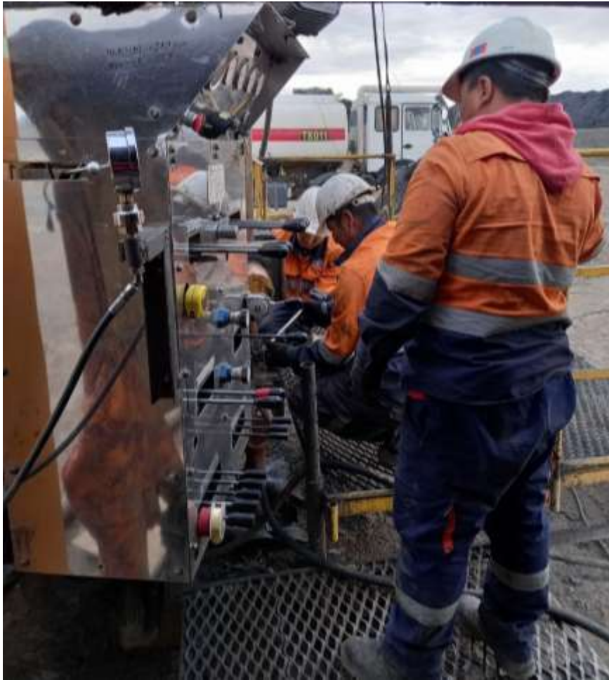
Figure 1 – Permeability testing being completed on the Snow Leopard - 03 well at the Gurvantes XXXV CSG Project in Mongolia
